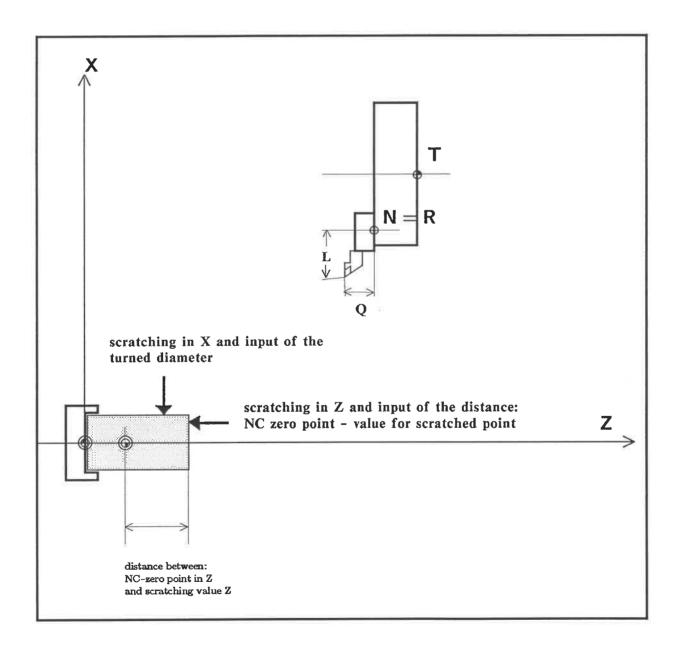
After the scratching process, the diameter reached by this is transferred to the control by actuating the ACCEPT NEW VALUE softkey and by entering the value of the diameter in digits. Since the NC zero point is identical with the machine zero point as far as the X direction is concerned, the value reached by scratching refers directly to the machine zero. Into the tool file is entered the difference between tool reference point N and the scratching value as presetter dimension L under address X.
