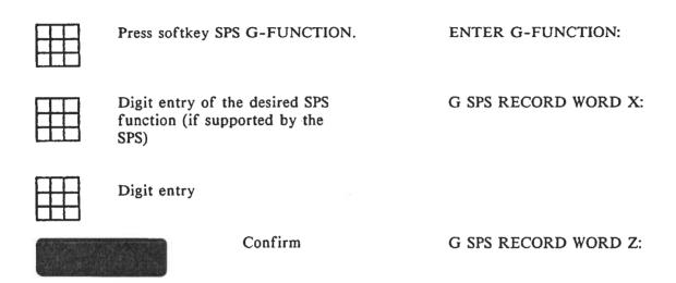
Proceed in a like manner when entering the other address parameters. If the last address parameter has been entered and/or confirmed, the function is evaluated by the SPS and the machine interface is configured accordingly Auxiliary programs for extensive movement sequences
