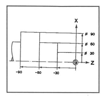
2. The dimensions indicate the distance from the previous point. This dimensioning method is called incremental dimensioning.
