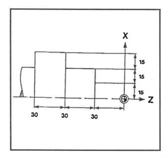
Depending on dimension data, target positions can be described to the control system by two methods:
