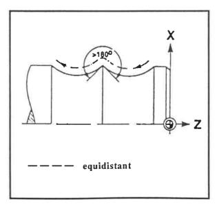
Cycles with tool nose radius compensation
