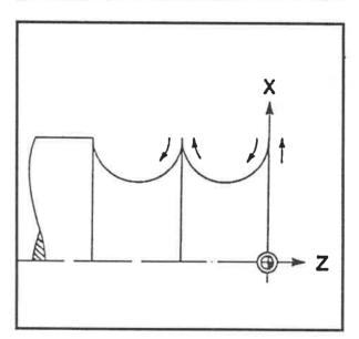
When tool nose radius compensation is active, the tool dimensions, including cutting edge radii, may not be altered.
