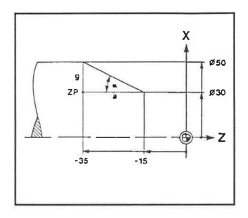
Longitudinal turning with straight adjoining contour and subsequent facing, LONGITUDINAL cycle, G81
