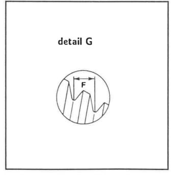
THREAD LEAD F: Thread lead in longitudinal direction
