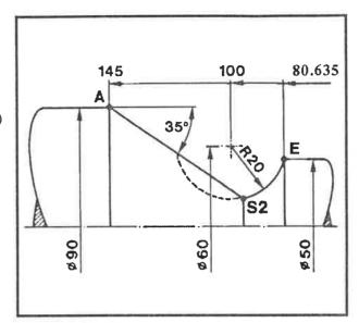
If intersection point S1 is desired, the circular arc must be programmed in two contour elements (e.g. K1, K2).
