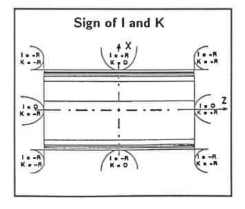
Programming instructions for G41/G42 In the block containing G41 or G42, only one straight line feed movement (G00 or G01) may be programmed. The actual point of intersection is taken into consideration from the next block onward.
