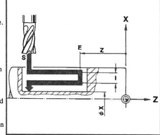
Before activating the cycle, feed in mm/min must be programmed with G94 and speed of the auxiliary drive with G197. Furthermore, the tool must traverse to a suitable starting point S which is located above one end point of the keyway.
