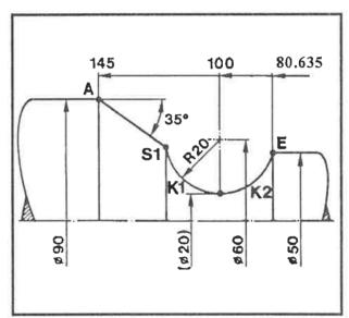
Circle-circle intersection point with non-tangential transition. The center points and radii of the circular arcs are known. Programming of such a contour will only remain error-free if start point A is entered or can be calculated. The point of intersection is
