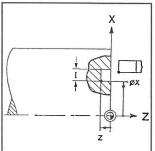
Axial groove with roughing and finishing:
