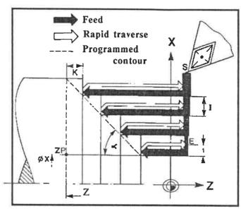
In contrast to the cycle illustrated on the last page this cycle does contain a programmed contour.
