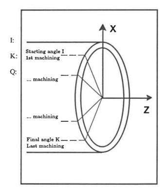
Example for programming the angle circle cycle First, five borings are machined by means of the drilling deep cycle and then a thread is cut. The drilling deep cycle is called up by means of a sub program while the threading cut is entered directly.
