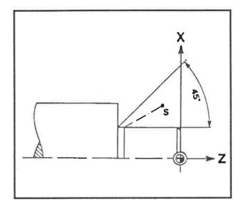
If SRK is being used in programming, the angle between the approach path and the following slanted section must be at least 180°.
