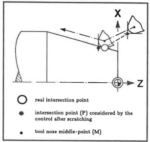
When tool nose radius compensation is active, no movements including a full reversal of direction may be programmed.
