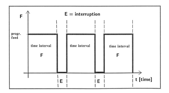
Switching the intermittent feed on and off The intermittent feed can be switched both on and off by programming the function G64.
