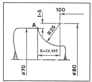
If start and end point of a contour element are not fully known, and if a point between them is known, it should be entered, whereby the contour element in question should be programmed in two parts.
