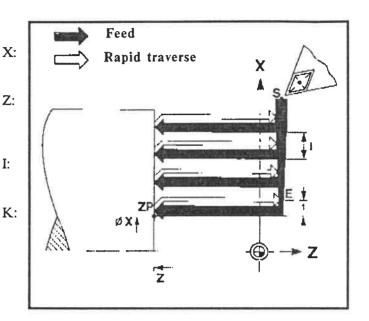
Longitudinal turning with straight adjoining contour, LONGITUDINAL cycle, G81 In this form of G81, steps are left on the adjoining straight line. There is no traversing to destination point!
