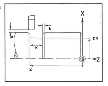
Groove with chamfers, roughing and finishing,
