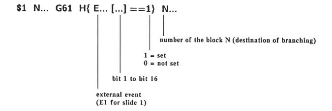
The table on the following page gives a survey of the function of the different bits in the external event E1. At this point events E2 to E5 have no meaning.
