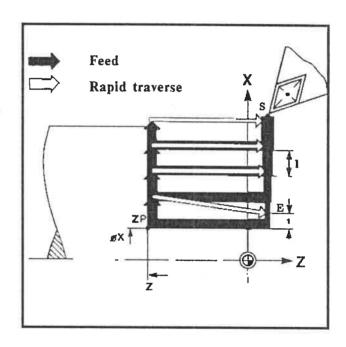
By means of I- (minus) a corresponding tool movement can be programmed even without a right-angled continuation.
