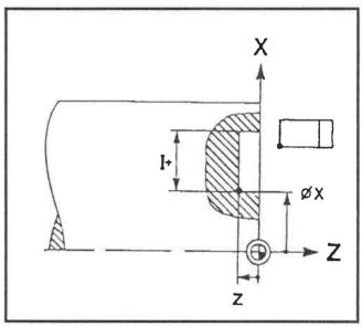
Axial groove G86 with chamfers
