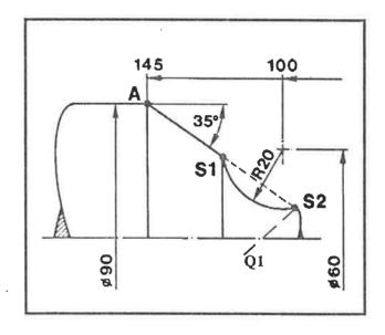
Each non-tangential transition must be programmed using B0. B0 is not necessary when: there is a transition between two straight lines, or when no destination coordinates have to be calculated in the preceding path, the current path and in the following path.
