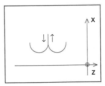
While the miller cutter radius compensation is active, the tool dimensions (X, L, Z), including the milling cutter diameter (D), may not be altered.
